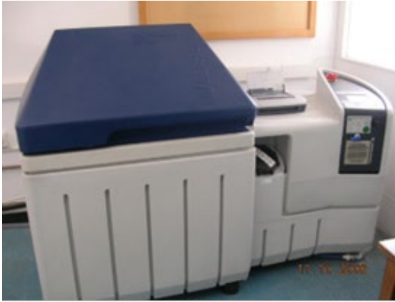
Figure 11. The salt spray chamber used is shown.
