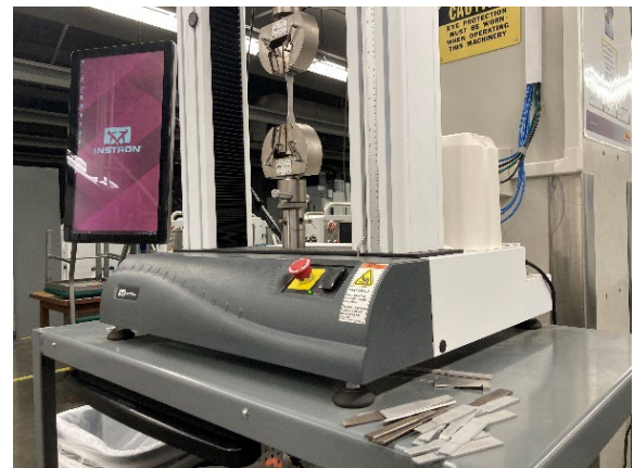
Figure 9. The computerized tensile test machine used is shown with AlSiC sample.
